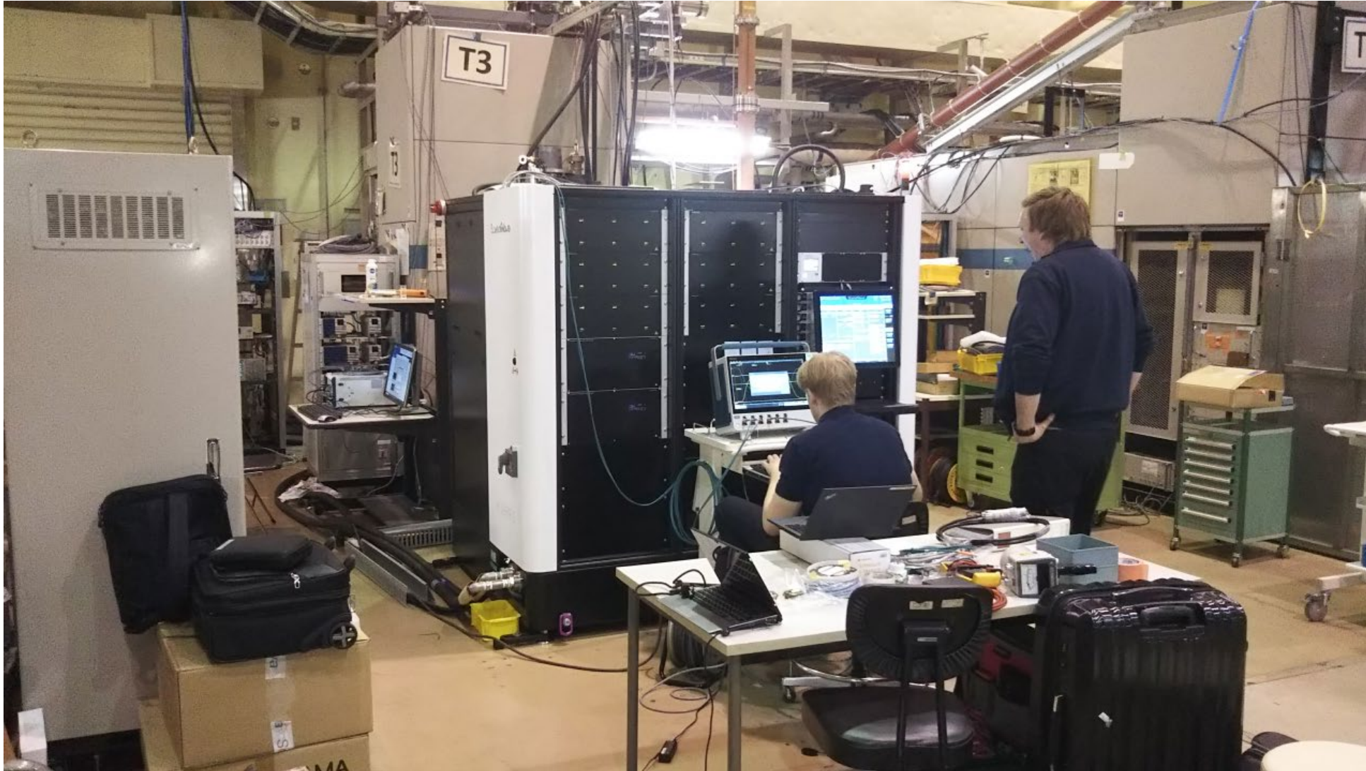
K-300 running at Test station T3, KEK Injector test hall. Achieving 40MW RF output power, Apr.17 2024. Now the station is under long-term running test.
