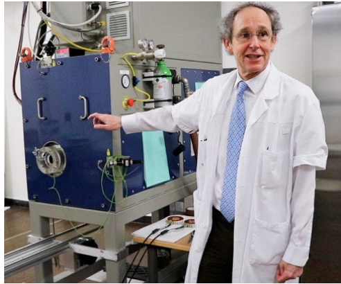
Experimental linac for FLASH radiotherapy manufactured by THERYQ (PMB-ALCEN) at CHUV
