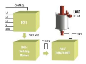
Fig. 1: The principle of the ScandiNova Solid State System
